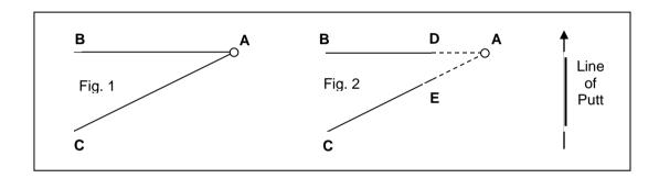
Before lifting the ball, two straight lines AB and AC are scratched in the sand as shown in Fig. 1. These lines should extend sideways from the ball. "A" is the marked position of the ball. When the smooth is completed, those portions of the lines represented by AD and AE in Fig. 2 will be obliterated. "A" can readily be located by projecting the lines BD and CE until they meet. The point of intersection will be "A" and the ball must be replaced on that spot.
